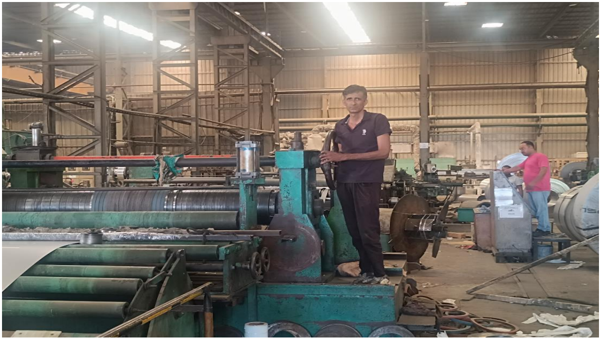
This is cold rolling machine used for decrease the thickness of the coil as per the desired output
