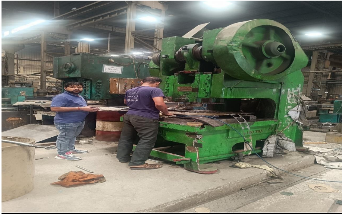
This is circle cutting machine used for cutting of circle used in utensil market.
