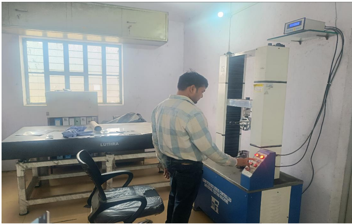
This is universal tensile machine, used to check the strength and longevity of the material.
