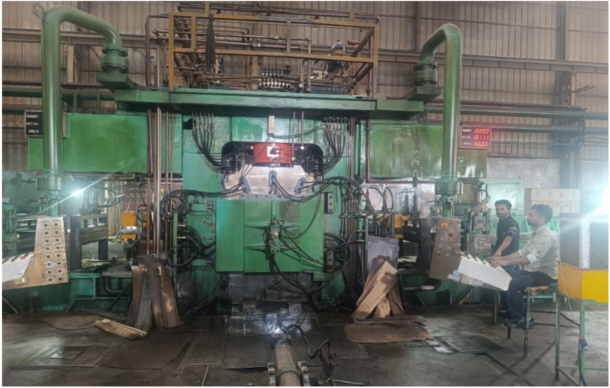
This is cold rolling machine used for decrease the thickness of the coil as per the desired output
